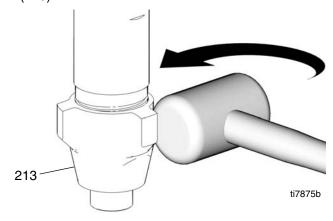
2. Disassemble and clean all parts and o-rings (207).
